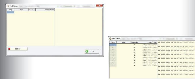
In this case, close this window, check the connection (see Step 17) and click again on the button «Test Timer». The test window opens, you can then transmit impulse timing data from the timer to the computer, then click on «OK».
